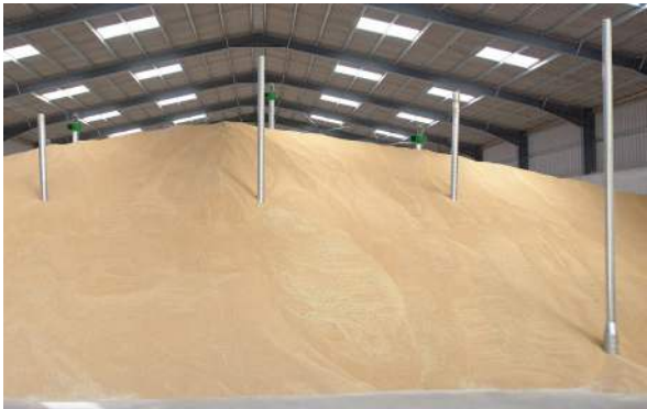
Pile-Dry Pedestals work in grain from 2.5m to 12m deep
