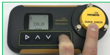
While the reading is visible, press Λ or V , the display will then show 0.0 , press ⓪ to display Grain Cell temperature.
