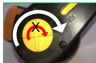
Ensure the yellow + remains stationary during grinding
